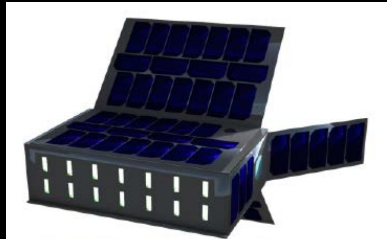
6U CubeSat with plasma thrusters
